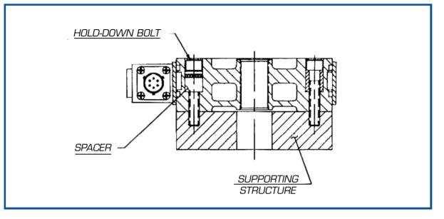
The purpose of spacers is to prevent loosening of Hold-Down Bolts.
