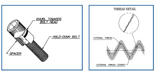
The longer the bolt, the larger the tightening elongation. In a short stubby bolt, loss of tightening elongation due to thread crumbling can be very serious. To reduce this effect to a manageable condition spacers are used. Spacers add to the length of the bolt, as well as provide some additional deflection themselves, and help maintain the desired bolt preload.
